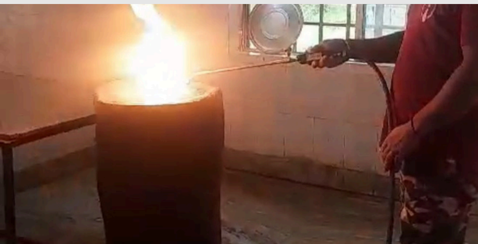
Fig: Disinfection of the surface of wooden chopping platform through blow flame application at Kitchen & Store
