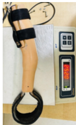
Carbon fibre prosthetic leg weighing 252gms
