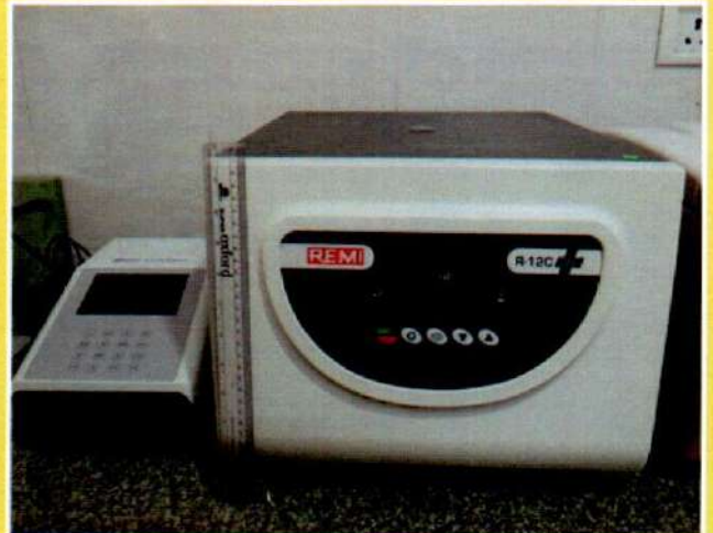
Hemocrit centrifuge machine for packed cell volume
