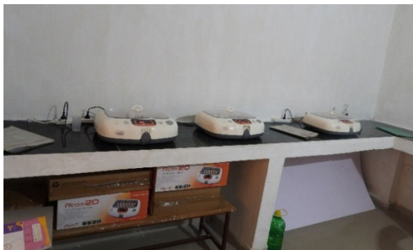
R-Com incubator used for artificial incubation of vulture eggs
