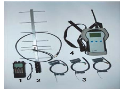
(vii) Radio Tag/tracker and receiver (For post-release monitoring)
