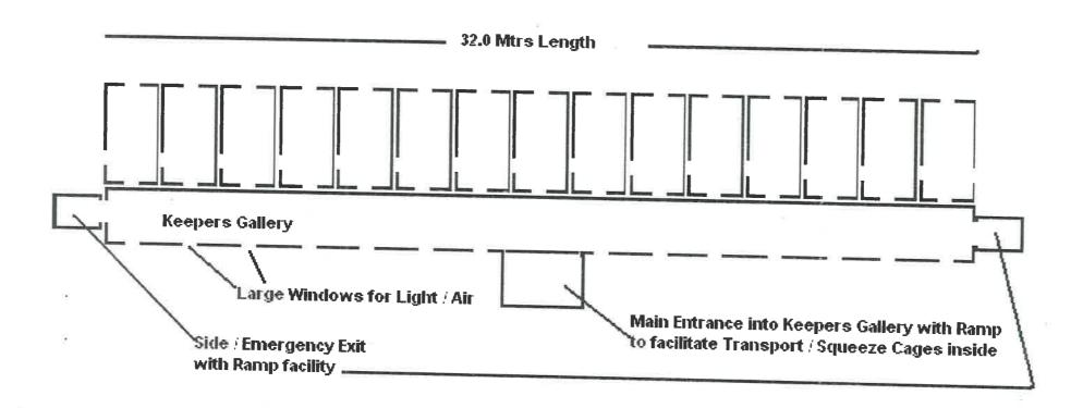
Top View of One 15 Den building unit structure
