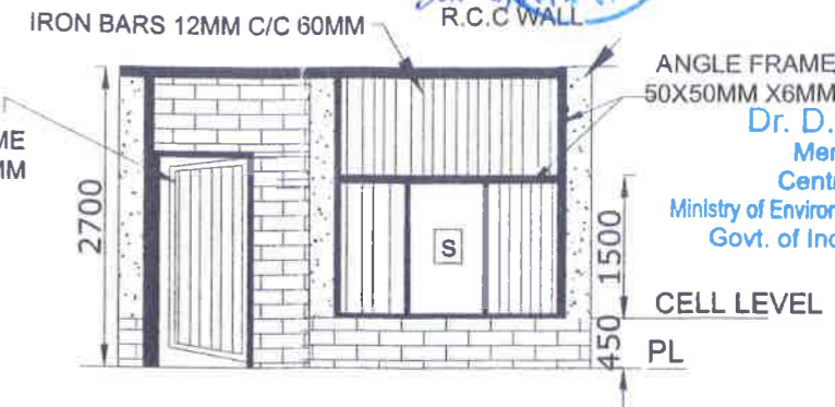
ELEVATION OF NIGHT CELL AT C-C
